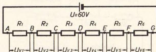
$$\begin{aligned} R_1 &= R_2 = R_3 = R_4 = R_5 = R_6 = 10 \Omega \\ R_g &= R_1 + R_2 + R_3 + R_4 + R_5 + R_6 = 60 \Omega \\ U_{v1} &= U_{v2} = U_{v3} = U_{v4} = U_{v5} = U_{v6} = 10 \text{ V} \\ U &= U_{v1} + U_{v2} + U_{v3} + U_{v4} + U_{v5} + U_{v6} = 60 \text{ V} \end{aligned}$$
